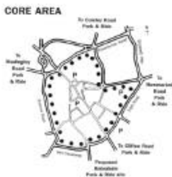
The Core Scheme aims to keep through-traffic out of the centre using a defined inner ring
